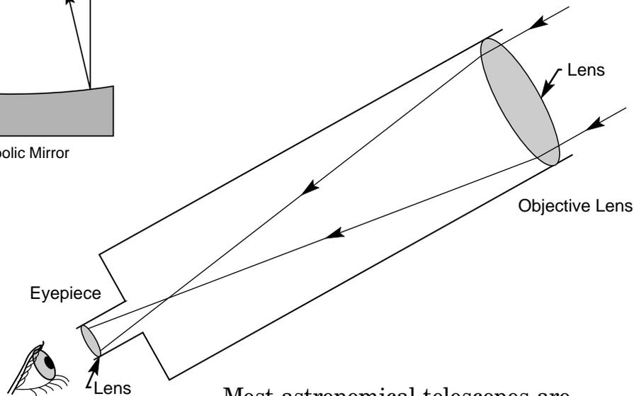
Most astronomical telescopes are reflectors. Objective mirrors are easier to make than objective lenses. Large mirrors are structurally easier to design and less expensive to build than large lenses.
