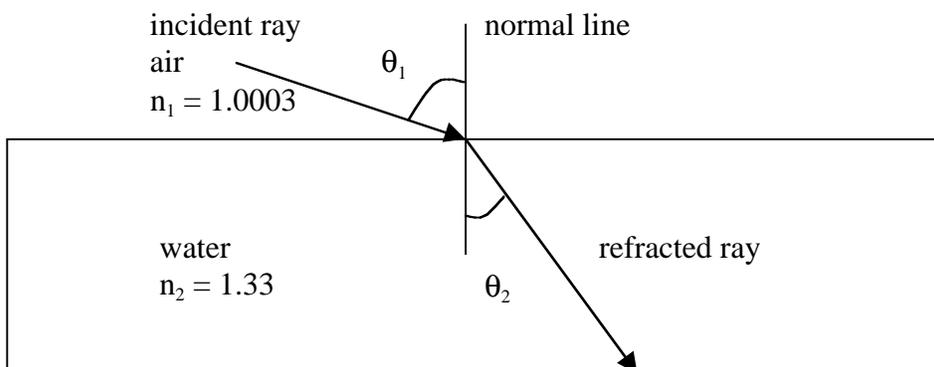
As an extension of Snell's Law note see Figure 2. Note how light will pivot towards the normal line when entering glass ( $n=1.5$ ) from air and then pivot back away from the normal line when exiting the glass block and returning to the air. Since the two glasses surfaces are parallel to each other, the incident ray and exiting ray are also parallel to each other with a slight lateral shift present.
