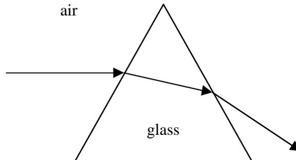
Figure 4 – Refraction of white light (or sunlight) through a glass prism. The range of dispersion is exaggerated for sake of clarity.
