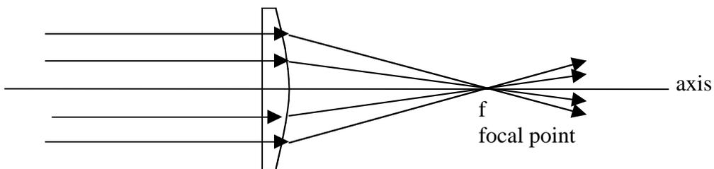
The path of light is reversible. Therefore light rays that pass through the focal point of and then strike the lens will exit in parallel paths. This is illustrated in Figure 6.
