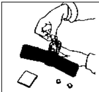
Leather pieces should be spaced evenly between the grooves. Be sure the leather gets good and wet with the glue.
