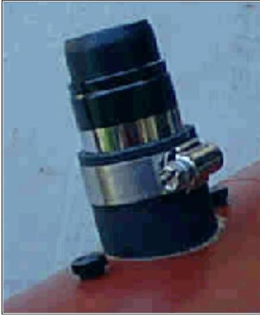
Gary Morris ([glmorris@jps.net](mailto:glmorris@jps.net)) came up with an elegant solution to attain the correct amount of "focusing friction": He simply uses a hose clamp (see photo at left)... He writes that it is a onetime affair to tighten the hose clamp around the cardboard focusing tube just enough to provide the necessary friction around the sink drain tube. (This would replace the need to "peel" or "glue in a strip of cardboard" in the two previous steps)
