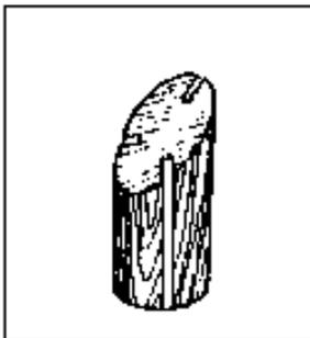
Dowel (closet pole, or handrail stock) with one end cut at a 45 degree angle. Three grooves should be cut (with a thin blade) at equal (120 degree) intervals (about 1/4" deep) as shown.
