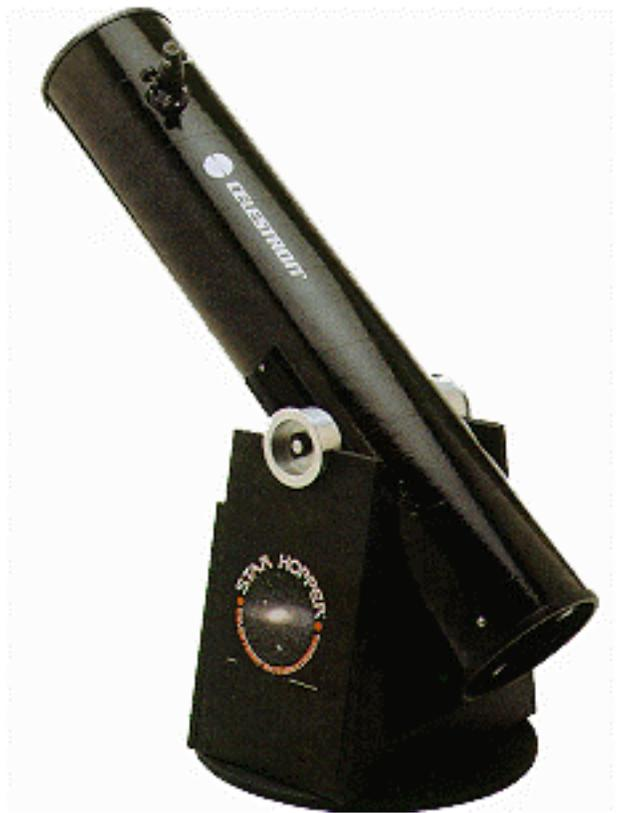
*Above: Celestron 8 inch f6 Dobson reflecting telescope, note simple Alt-Az mount. Courtesy Celestron.*
