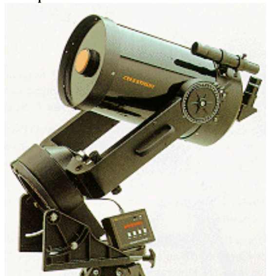
Above: Celestron 8" Schmidt-Cassegrain telescope on Fork Mount, Equatorial Wedge. Courtesy Celestron.
