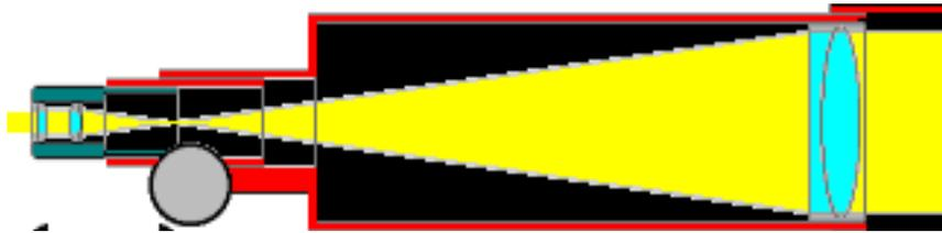
**A typical refracting telescope**
