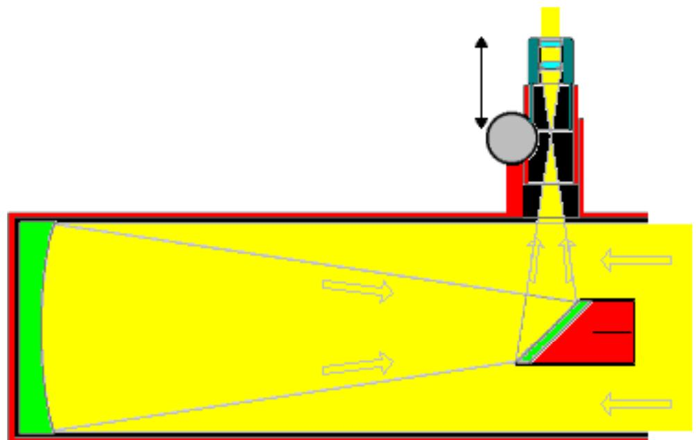
A typical reflecting telescope
