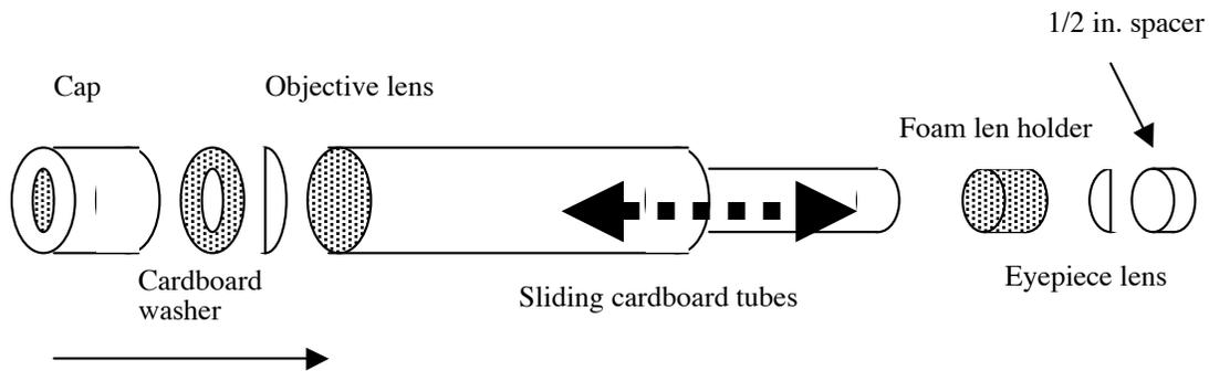
Some words about the basic operation of a simple telescope. The objective lens (long focal length) collects light from a distant object, and forms a small, upside-down image near the focal point. The eyepiece lens (short focal length) then acts as a simple magnifier to enlarge this small upside-down image. The tube of the telescope is only a physical support to make sure the lenses remain in proper relationship to each other.
