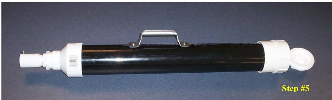
To complete assembly, add a garage door handle (part 14) to the top of telescope. Pick a handle that is constructed so that it is formed in a tube where you grasp it. Be careful to align it along the length of the telescope. The telescope tubes have writing imprinted along their length, which can be used to align the handle. With this type of handle and proper alignment, you will not only have a convenient way of carrying your telescope but a finder sight as well.
