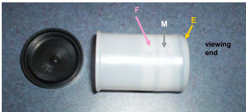
**Image #3:** Completed eyepiece assembly
